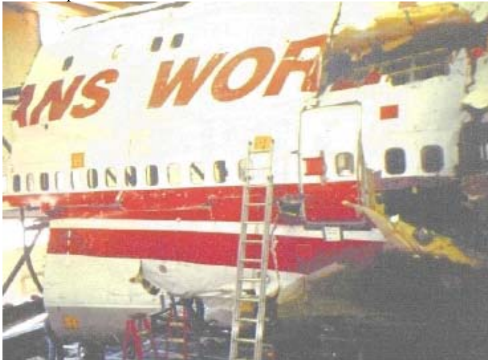
The left front of the reconstruction at LF4
